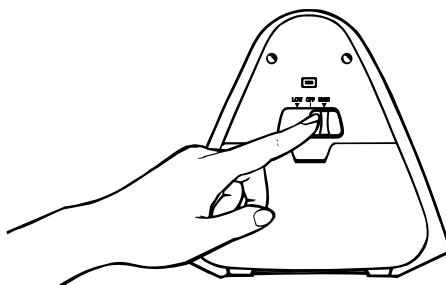
To start swing, slide the speed button to the desired speed and give the swing a gentle push. Red light comes on when swing is turned on.
